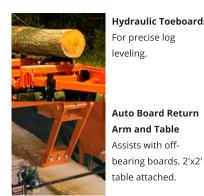
**Hydraulic Toeboards** For precise log leveling.
