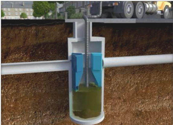
Fig.2 Maintenance is performed with a vector truck.
